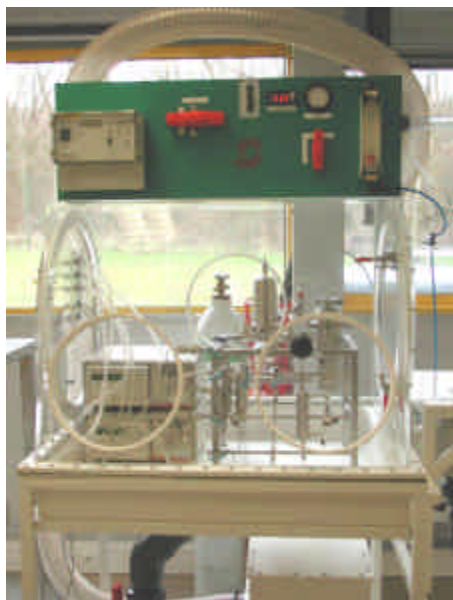
Figure 1 : New chemical entities process screening equipment placed in an isolator
