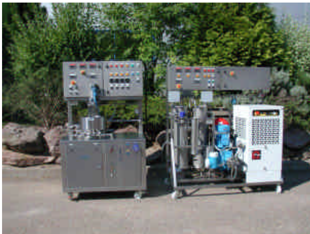
Figure 2: “Ultra clean” 7-litre pilot scale equipment designed in 2 skids to be placed in a “grey” room (pumping, heating, vent) and in class B environment for the main particle formation vessel.
