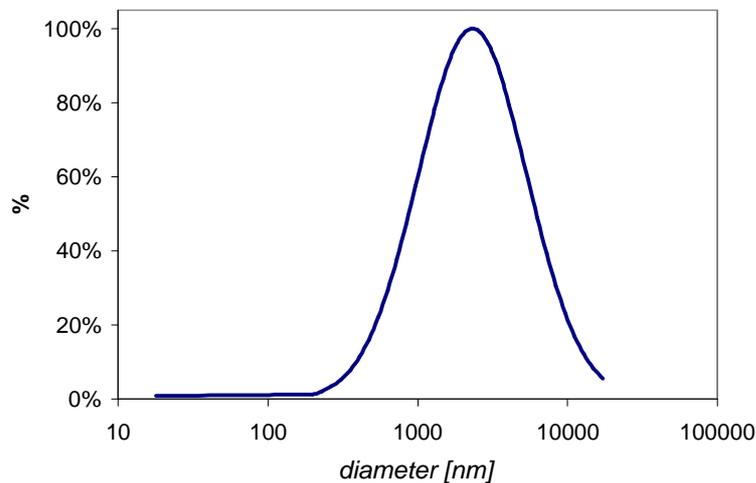
**Figure 4:** Particle size distribution of tristearin/phosphatidylcholine (50:50 w/w) micro-particles obtained at 20MPa, 333K, 180  $\mu\text{m}$ -nozzle.
