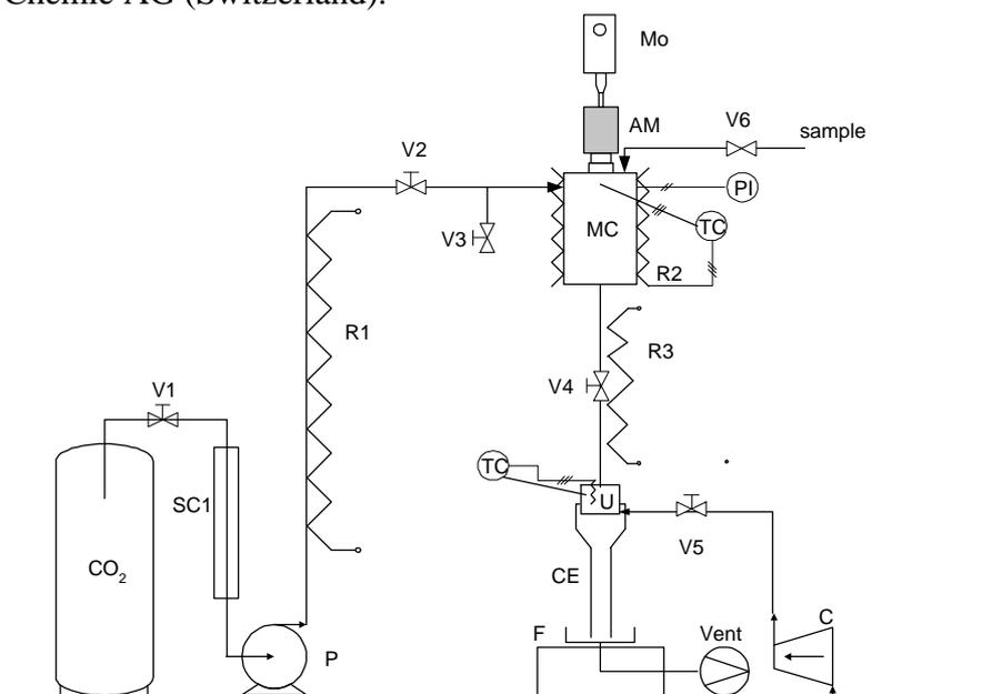
**Figure 1:** Schematic of the PGSS set-up: MC: mixing chamber; U: nozzle; CE: expansion chamber; F: filter; Mo: engine; AM: magnetic mixer; R1, R2, R3 e R4 resistances; SC: heater exchanger; P: CO<sub>2</sub> high pressure pump; V1, V2, V3V4 and V5: on-off valves; PI: pressure gauge; TC: temperature control.
