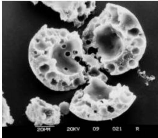
**Figure 3:** Fractured micro-particles of tristearin obtained by PGSS
