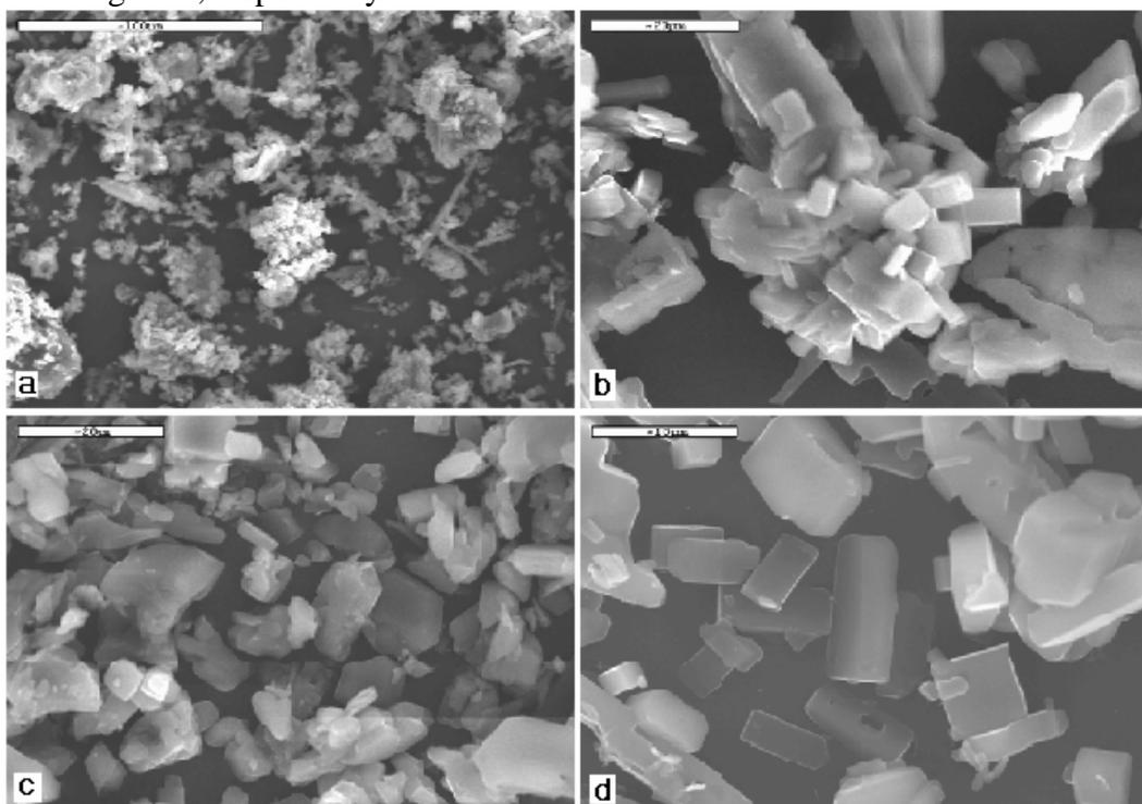
**Figure 3.** SEM microphotographs of Paracetamol particles processed at 40 °C, 4 w/v % concentration and at a)100 bar, b)150 bar, c)200 bar, d)250 bar
