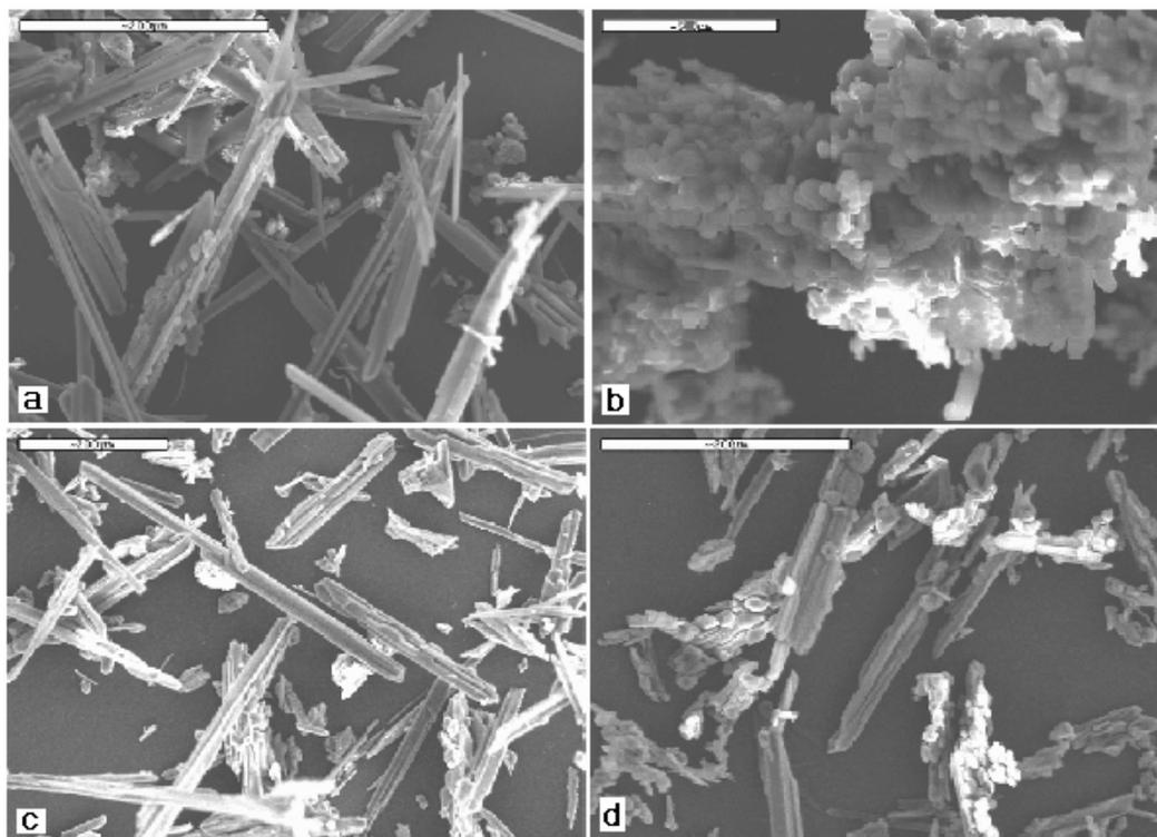
**Figure 2.** SEM images of processed Paracetamol particles at a)150 bar and 60 °C, b)150 bar and 80 °C, c)250 bar and 60 °C, d)250 bar and 80 °C
