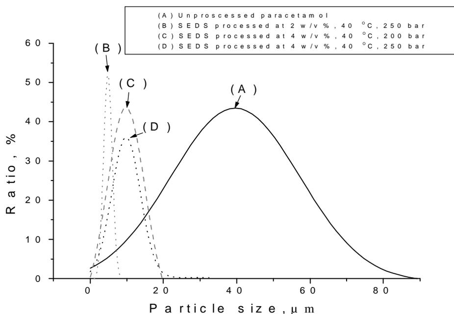
**Figure 4.** Particle size distribution of unprocessed Paracetamol (A) and SEDS processed at: 2 w/v %, 40 °C , 250 bar (B); 4 w/v %, 40 °C , 200 bar (C); 4 w/v %, 40 °C , 250 bar(D).
