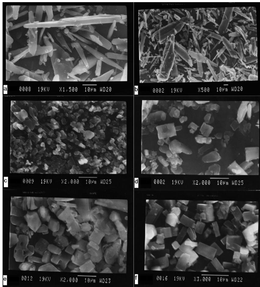
**Figure 1.** SEM images of unprocessed Paracetamol particles a), b) and processed Paracetamol particles at 40 °C at c)100 bar, d)150 bar, e)200 bar and f)250 bar
