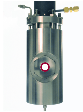
Figure 4: View cell used for the the magnetic suspension balance
