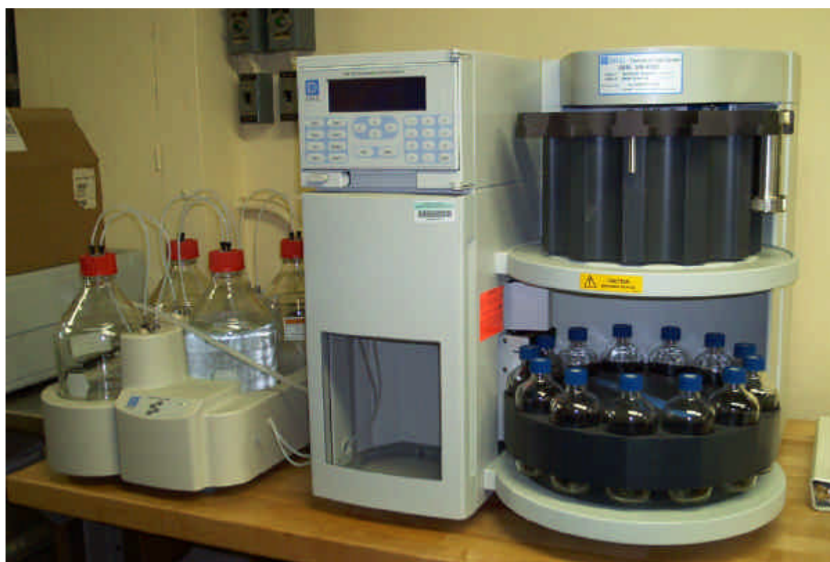
Fig. 2 Accelerated solvent extraction module (Dionex Model 300) used for the SWE of fruit berry substrates.
