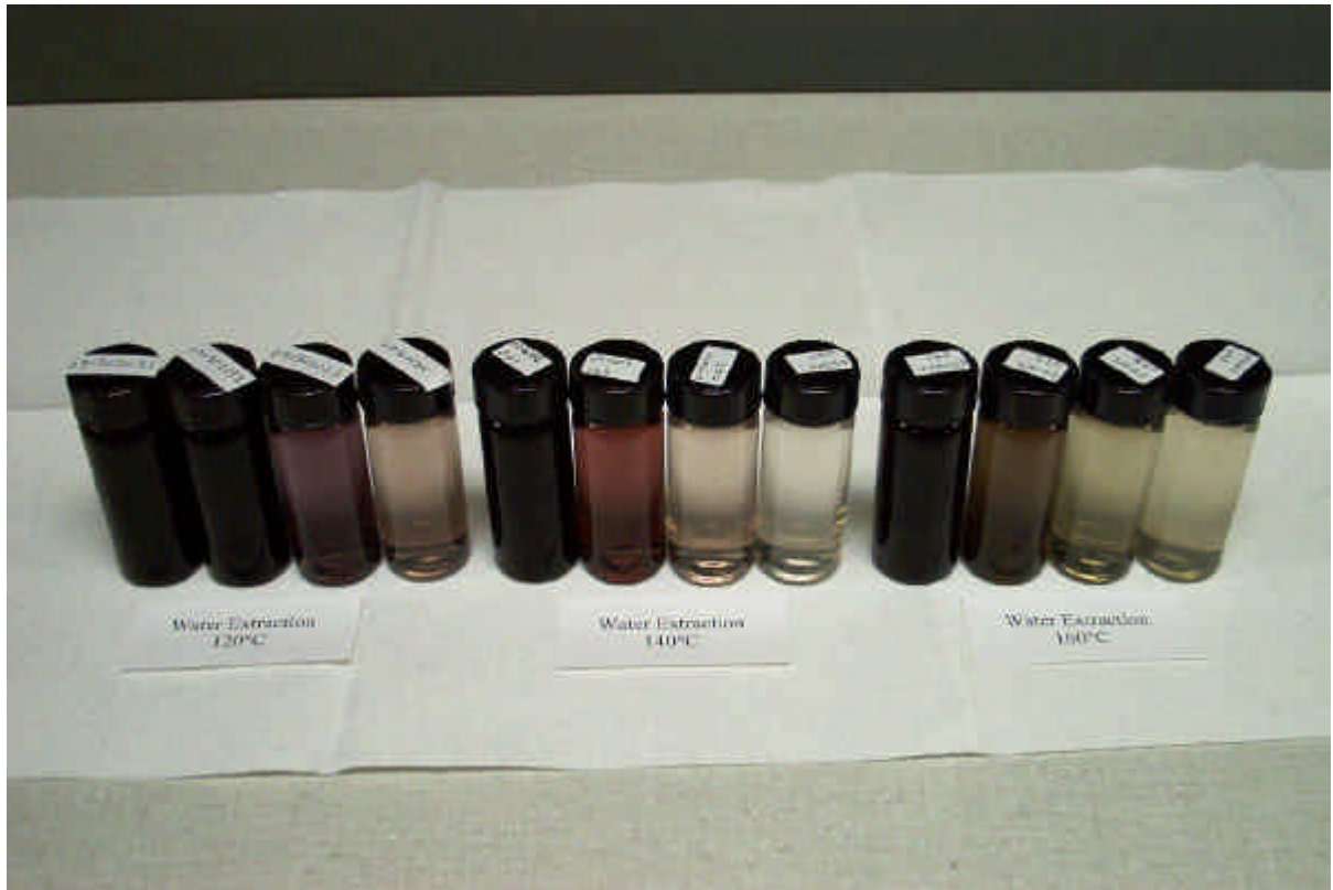
Fig. 3a SWE of elderberry pomaces using degassed water as a function of temperature.
