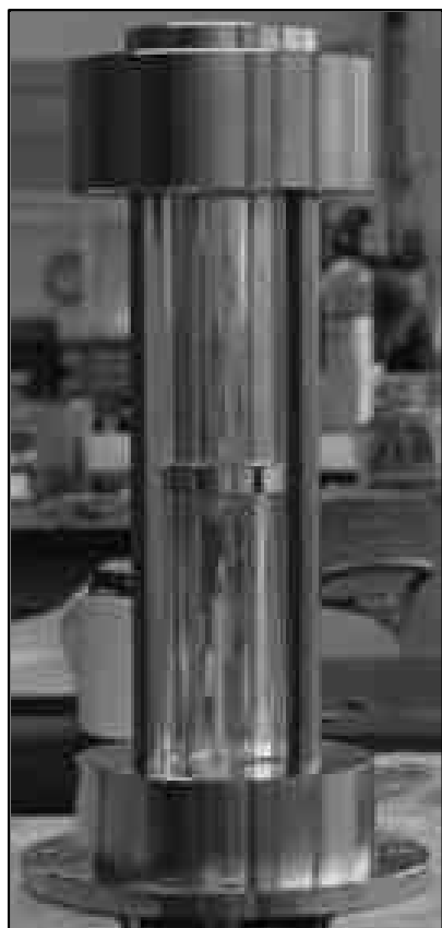
Figure 2 : Transparent vessel for phase equilibrium measurement.
