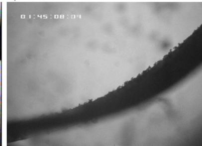
**Figure 4:** Surface (in this case: PTFE) prior and after hydrate formation.  $T_a = T_0 = 285$  K,  $p_a = p_0 = 20,0$  MPa,  $w_{\text{H}_2\text{O}} = 0,14$  wt-%;  $T_b = 275$  K,  $p_b = 11,5$  MPa,  $w_{\text{H}_2\text{O}} = 0,095$  wt-%;  $T_c = 273$  K,  $p_c = 9,8$  MPa,  $w_{\text{H}_2\text{O}} = 0,085$  wt-% (The water content is estimated according to figure 7)
