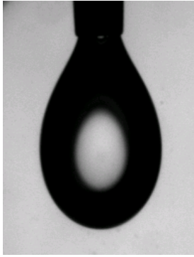
Fig. 4: Drop of water in supercritical \text{CO}_2 (10 MPa, 308 K)
