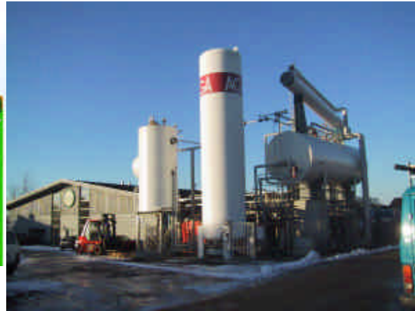
Figure 4. The world's first commercial supercritical wood treatment plant – CO 2 storage, separation and recovery system
