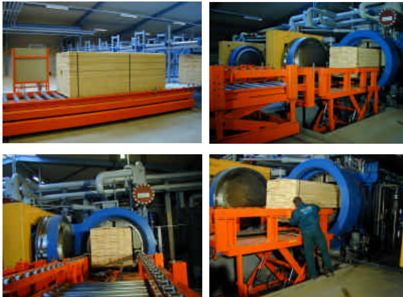
Figure 5. The world's first commercial supercritical wood treatment plant – receiving and handling system.
