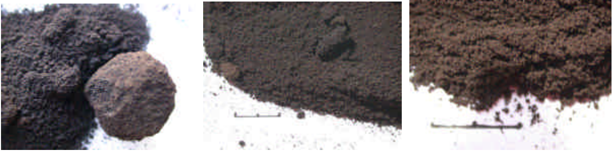
(a) 4.0MPa (b) 4.5MPa (c) 5.0MPa Figure 2 Apparent states of fine asphaltene particles (Full scale= 1cm)
