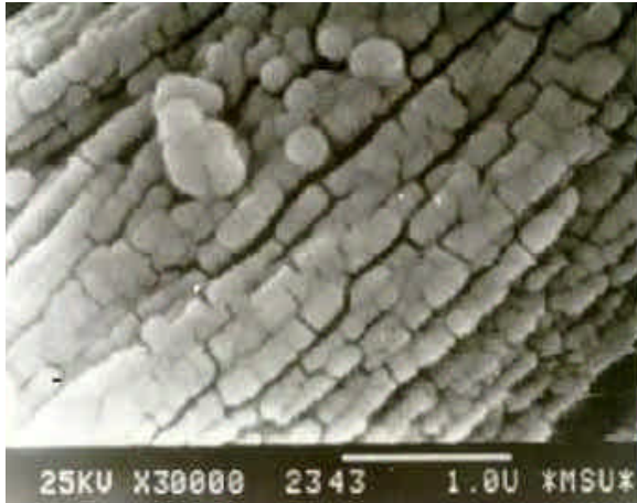
Figure 6. The intermediate fibrous phase silica predecessor of keatite.
