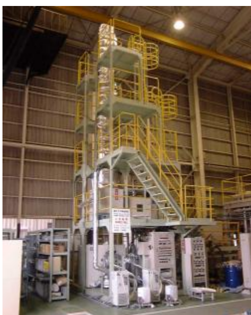
Fig.6 The continuous depolymerization apparatus
