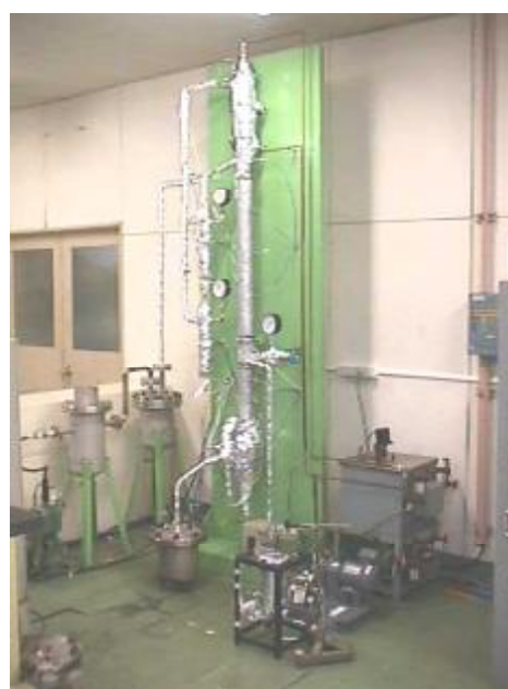
Fig.7 The continuous distillation apparatus
