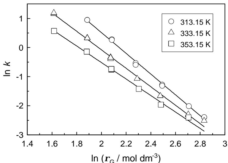
**Figure 1.** Retention factor of naphthalene as a function of mean molar density of CO<sub>2</sub>. Open tubular column (4.20 m × 85 μm i.d.), [bmim][PF<sub>6</sub>] film thickness 0.16 μm.
