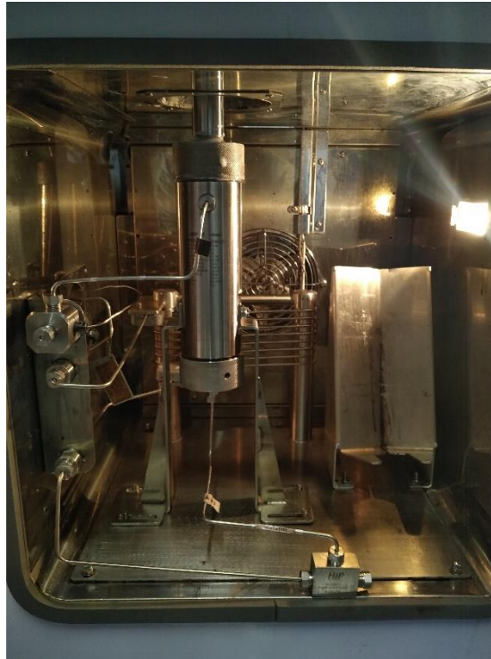
Autoclave 100mL – 1000 bar 150C (CO 2 ) ~250 bar 150C (eau)
